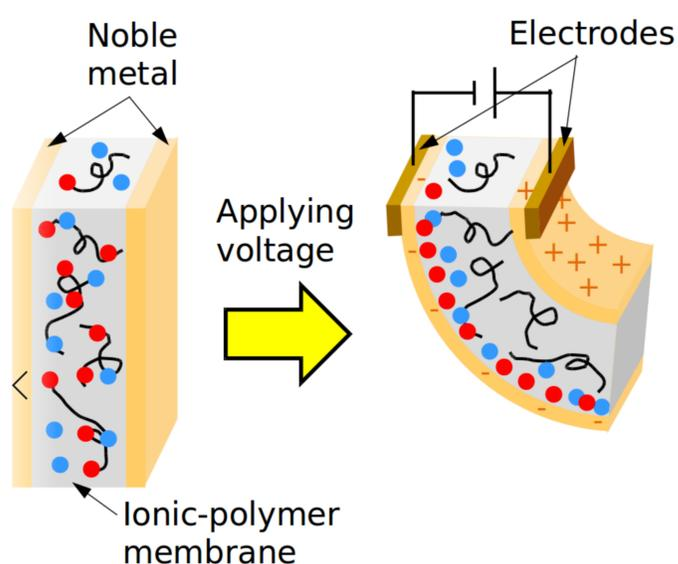
Figure 2: Functional principle of an ionic EAP performing a bending motion once voltage is applied.
