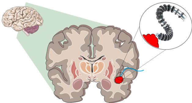
Figure 1: Utilisation of a snake-like instrument to approach a lesion in the human brain avoiding damage to non-involved tissue. Source: MTU Aero Engines (modified).
